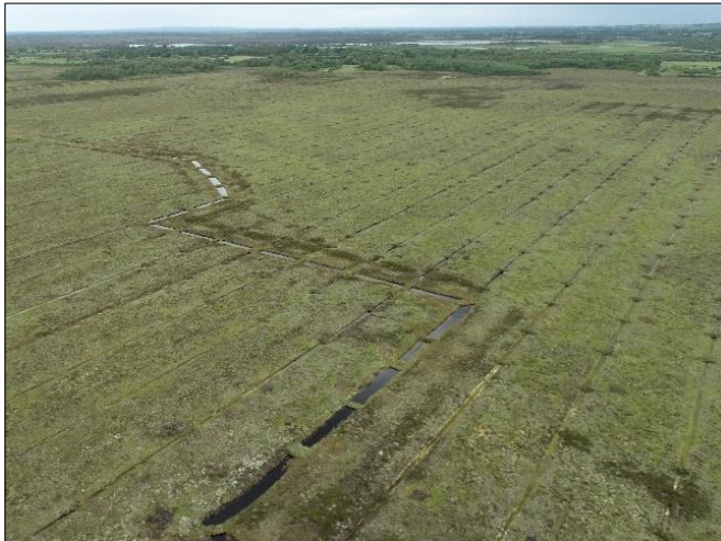
Plate 3.3 Drone photo of Killeglan bog with former drains blocked in this area. Some additional targeted drain blocking has been identified to increase the extent and resilience of former drain blocking.
