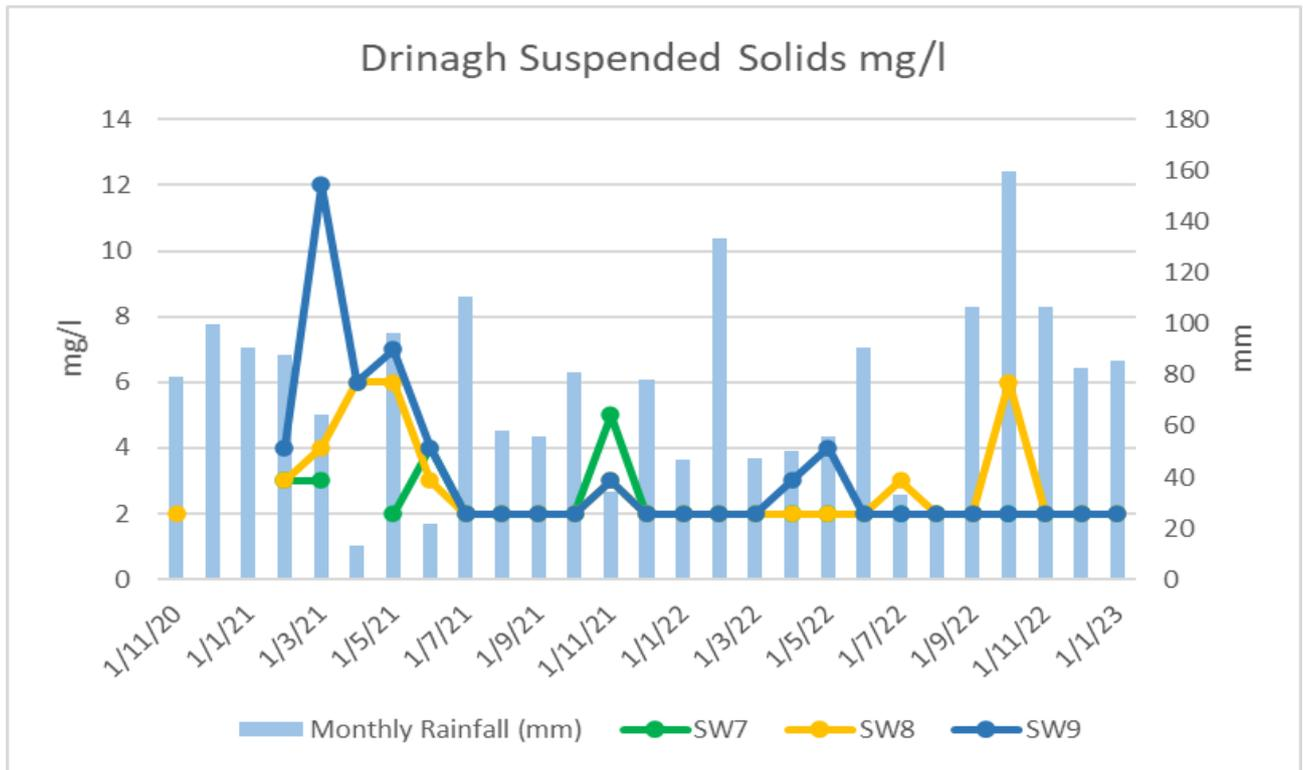
Figure AP13.1. Suspended solids in water sampling at Drinagh from different discharge points. 35 mg/l is the emission limit value.
