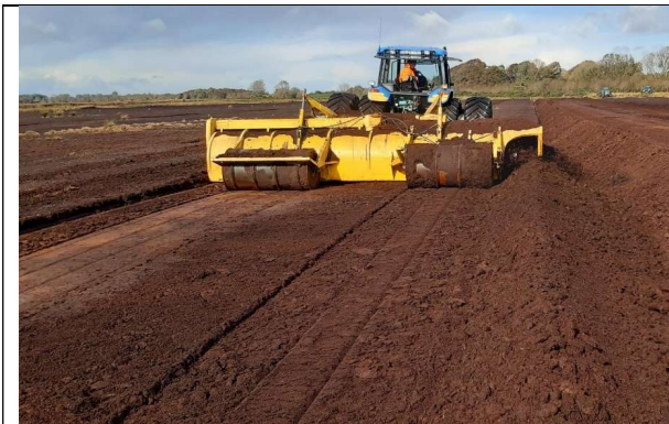
Figure 7.5. Screw-leveller removing the camber of peat-fields at Castlegar Bog.
