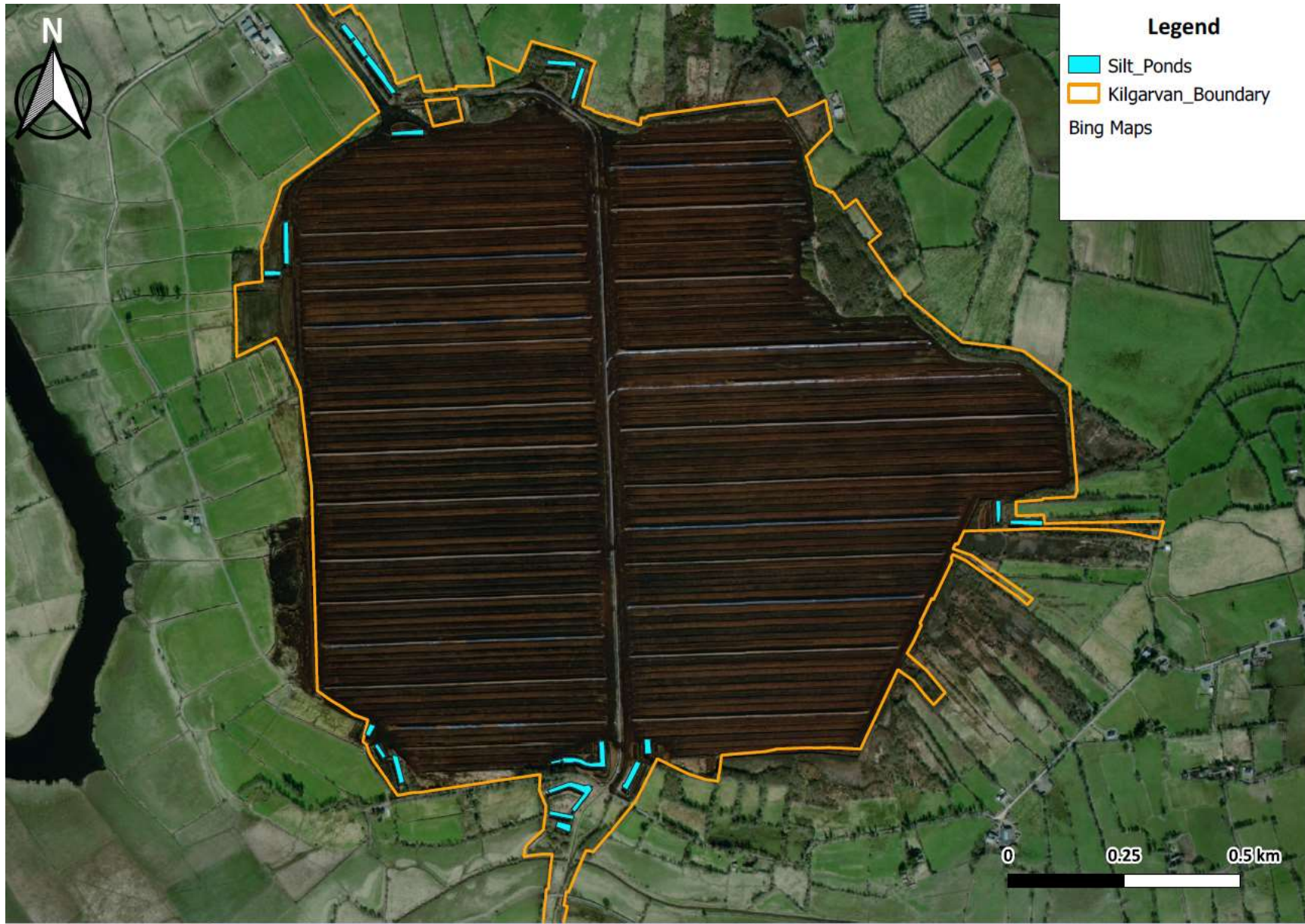
Figure 21: Kilgarvan Bog Site Drainage and Silt Ponds
