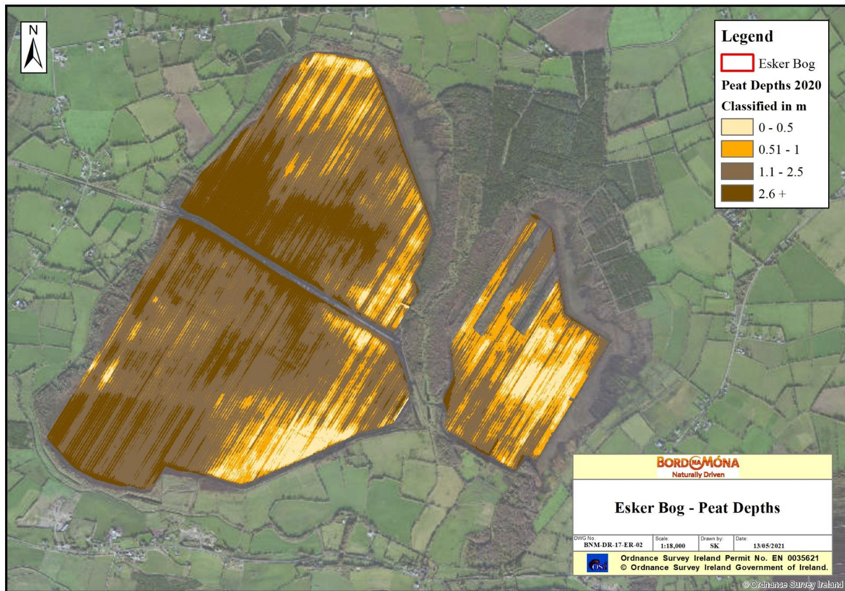
Figure 8.2. Peat Depth Map for Esker Bog (2020). There are pockets of deep residual peat (western area); the remainder is shallow cutaway.
