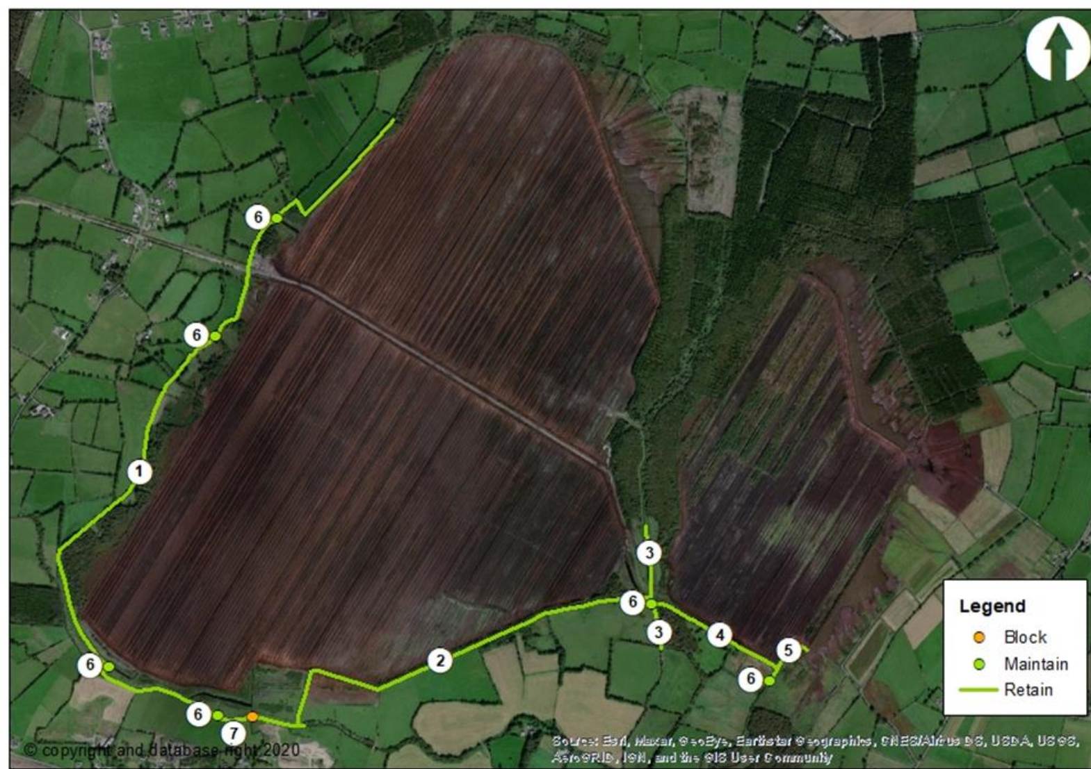
Figure 11: Drainage Management Measures for Esker Bog (derived from the Drainage Management Plan for Esker Bog)
