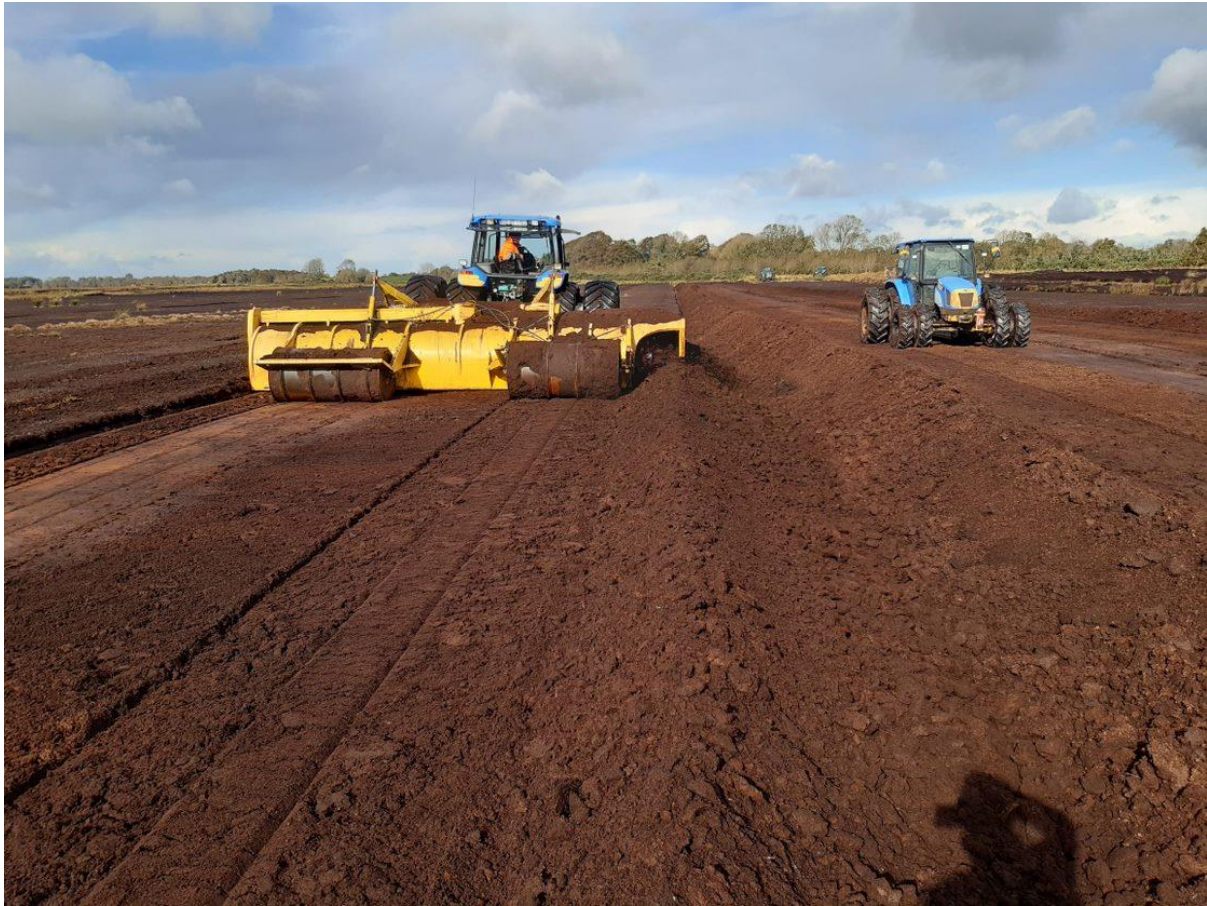
Figure 5.4.1 Field re-profiling using Screw-Leveller
