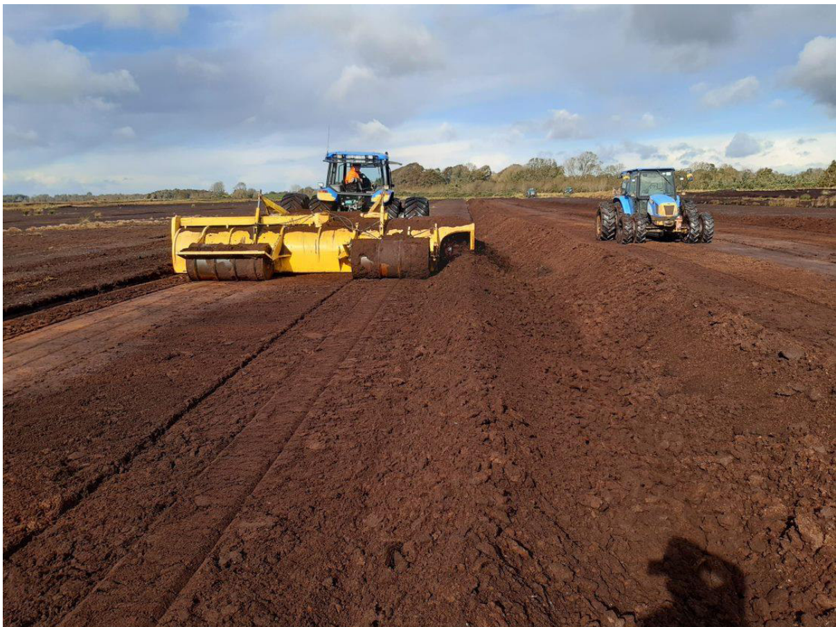
Figure 5.5.1 Field re-profiling using Screw-Leveller
