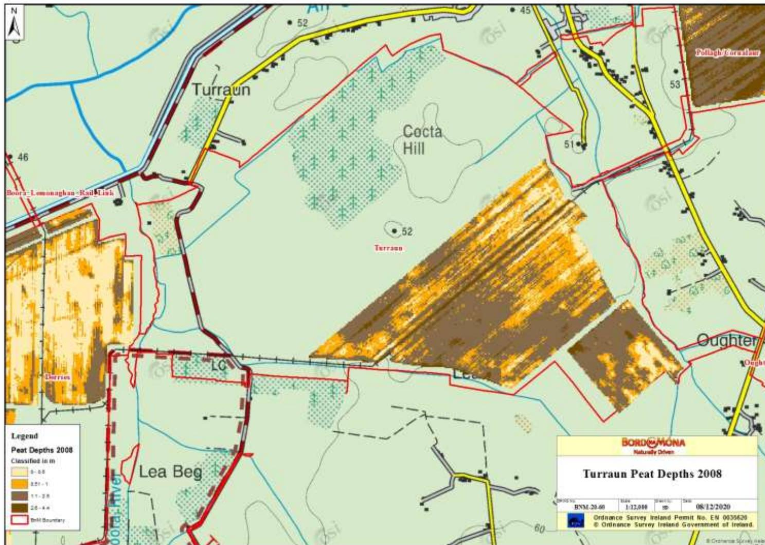
Figure 8.2. Peat depth (2008) map for Turraun Bog. Data is not available for the western side as it was cutaway
